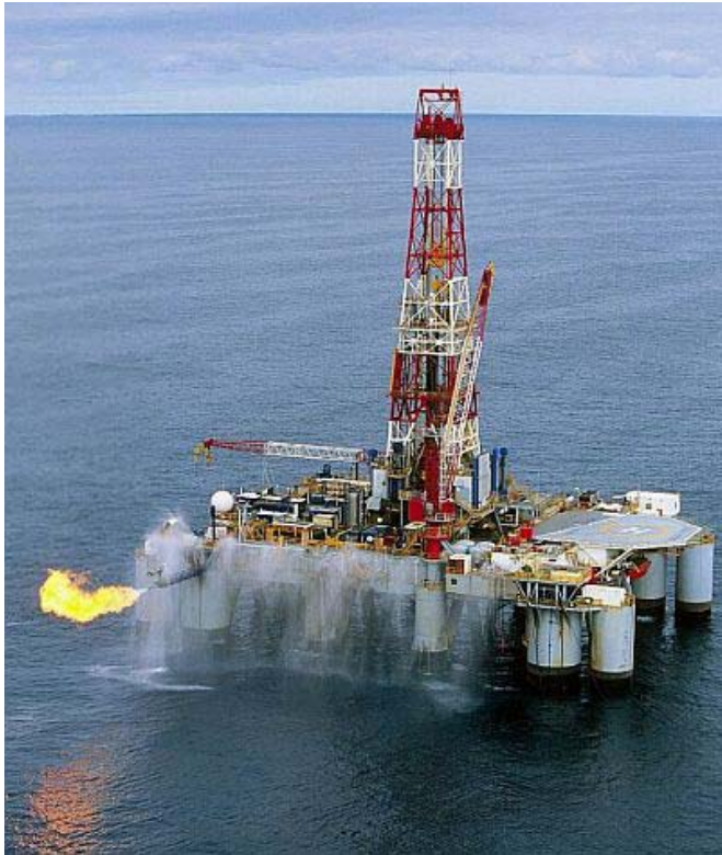
The Ocean Epoch semisubmersible drilling rig.
